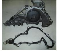
Both pumps to the left were supplied with a metal gasket with a rubber lining the interior perimeter. This type of gasket does not require any sealer. It is clear that over use and misuse of sealants occured. Installation practices of this nature will lead to premature water pump failures. Premature failures lead to product reliability / quality concerns from customers when in actuality the failure arose from miss-installation / improper use of sealants.
