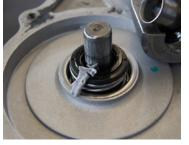
To the left are examples of Dynamic and Static seal contamination / filming caused by over use of sealants. When sealant particulates / residue get trapped between the Dynamic and Static seal faces it causes a separation of the two surfaces which leads to a seal leak.
