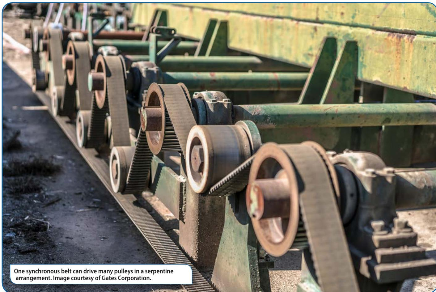
One synchronous belt can drive many pulleys in a serpentine arrangement. Image courtesy of Gates Corporation.
